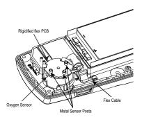
Gently remove the circular rigidified flex PCB atop the sensor from the metal sensor posts. Take care not to tear the flex cable. Note the placement of the PCB to ensure it is replaced correctly. Remove the two screws on the PCB.
